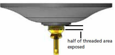
Drawing 2 – Canopy Adjustment
